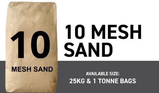
10 Mesh Sand is a general purpose course sand that's commercially dried and screened. It is used for mortars and plasters, concrete sand, drainage and filtration. In general, it has a top particle size of 2.36 and a bottom particle size of 0.75um.
